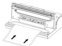
Clean and straighten the open end of the bag--ensure there are no wrinkles or ripples.
