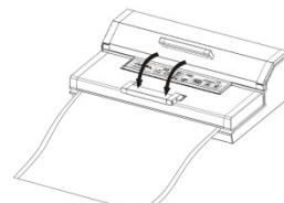
Put one end of the bag on top of the sealing profile, but not enter the vacuum chamber.
